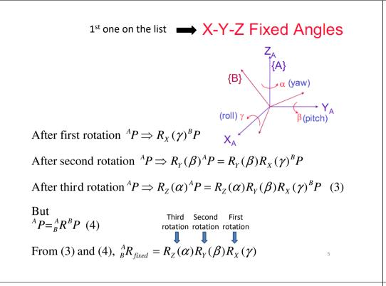
Euler Angle Rotation  $R_Z(\alpha)R_Y(\beta)R_X(\gamma)$
